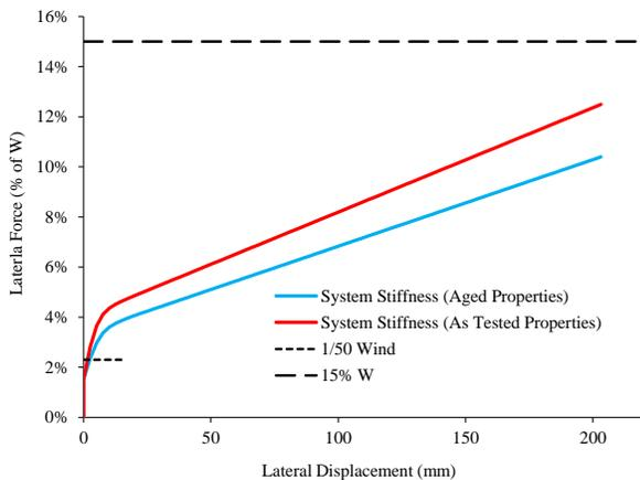
Figure 4. Force displacement properties of LRBs – As-Tested and Aged Properties.
