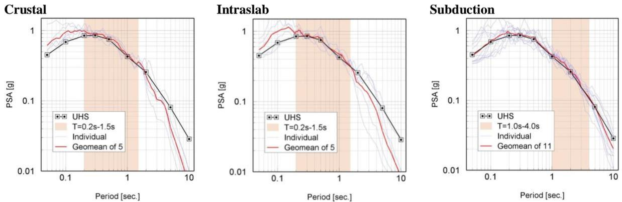
Figure 3. Horizontal component geometric mean (Geomean) relative to the UHS for the three different suites, scaled to be at or above the UHS in the applicable period range (note colour band shows period range for selection only; scaling for Crustal and Intraslab done for period range  $T=0.5$  to  $1.5$  s; scaling for Subduction as shown for period range  $T=1$  to  $4$  s).
