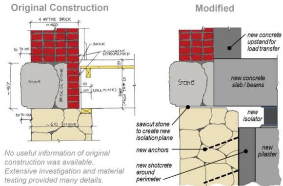
Figure 7. Comparison of Exterior Wall before and after isolation work completed.
