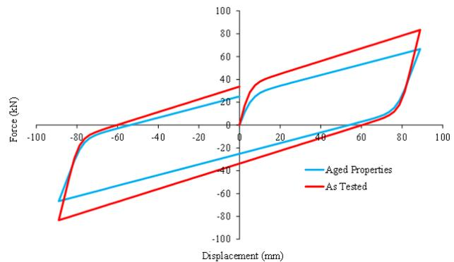
Figure 5. LRB test cycle to evaluate energy dissipation.
