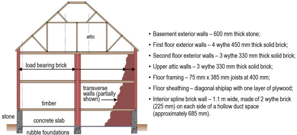
Figure 1. Cross section of original structure and description of elements.
