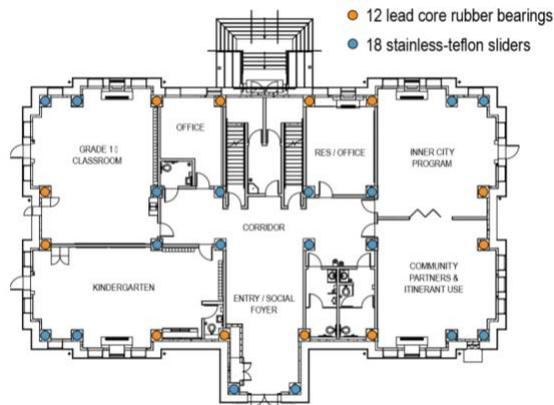
Figure 6. Basement plan showing locations of bearings and sliders.
