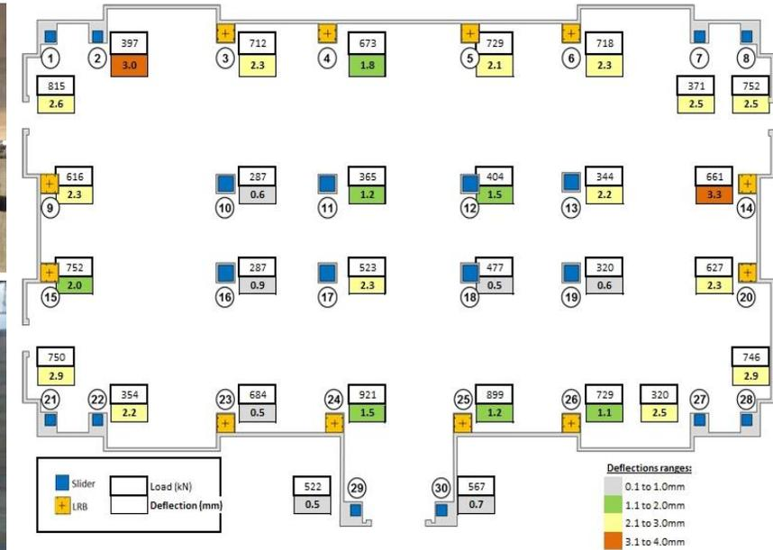
Figure 10. a) View of slider during jacking (left, top) b) Slider location atop column, shoring in place (left, bottom) c) Force-Deflection summary after load transfer complete.
